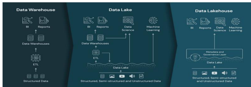
Figura 4. Data Warehouse, Data Lake, Data Lakehouse. Fuente: Ben Lorica, Michael Armbrust, Reynold Xin, Matei Zaharia y Ali Ghodsi. What Is a Lakehouse? https://www.databricks.com/blog/2020/01/30/what-is-a-data-lakehouse.html
